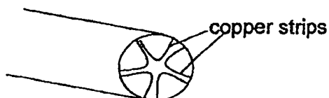
copper pipe B lined with copper strips
